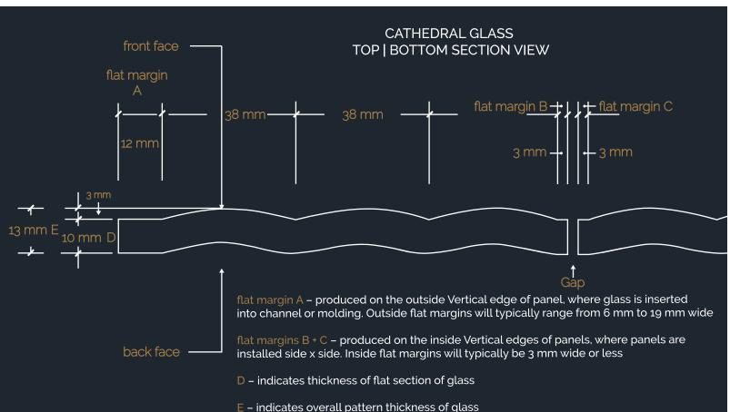
(Please note that the pattern thickness depth can vary slightly, from 2mm to 4mm, on some panels)
